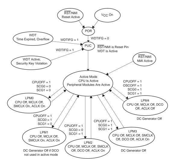
Figure 2–10. MSP430x1xx Operating Modes For Basic Clock System
